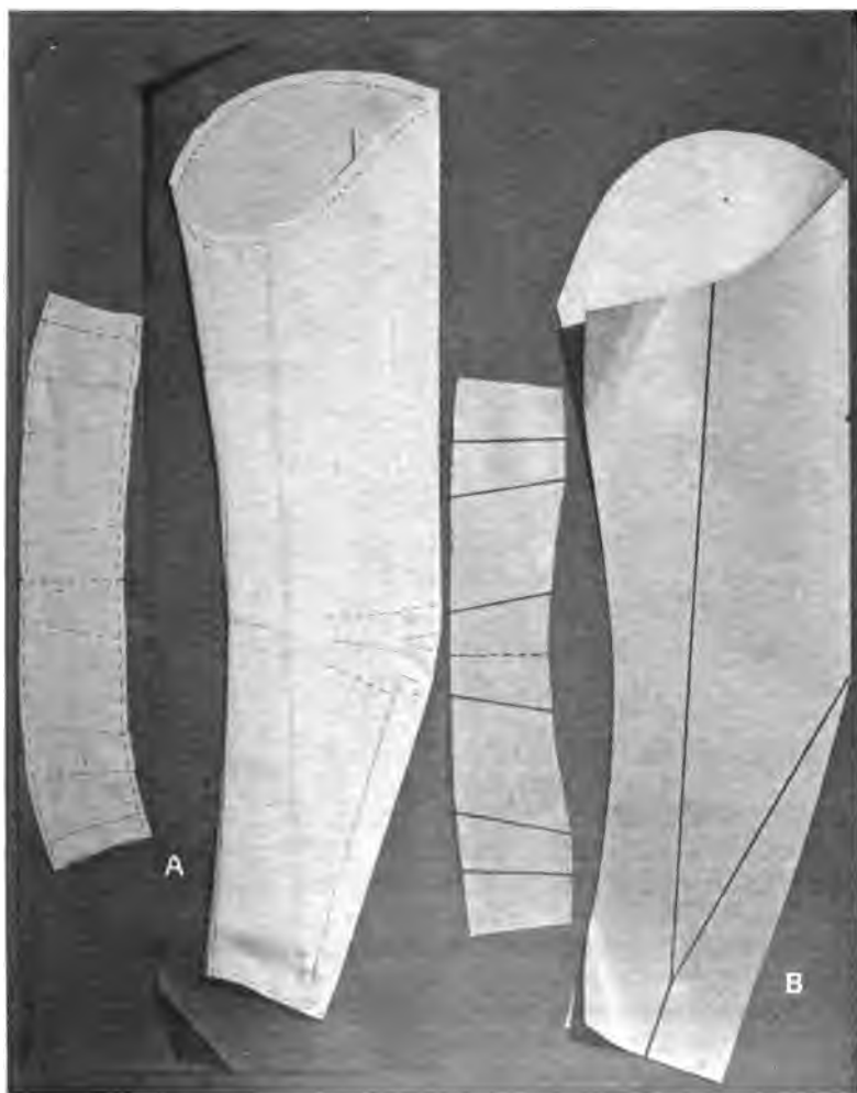
FIG. 81.—Making cardboard sleeve and collar; A, sleeve lining placed on folded cardboard; also muslin collar; B, cardboard sleeve cut out and marked; collar board also.
